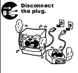
Continued use of the machines in an abnormal condition such as when the machines are producing smoke or strange smells may cause **fire** or **electric shock**. In these cases, immediately turn off the power switches and disconnect the power cord plugs from the outlet. Then, contact your authorised TOSHIBA TEC representative for assistance.
